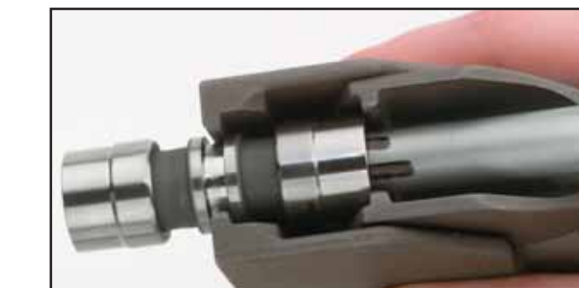
To swage the fitting, apply pressure. Upon completion of swaging, release the pressure, the moveable jaw will return to the original position.
