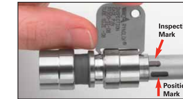
Visually inspect that the ring is fully advanced onto the fitting using the Rynglok® Inspection Gauge (P/N: RTSG0-51-XX). Be sure to verify that the edge of the fitting is within the limits of the inspection mark.
