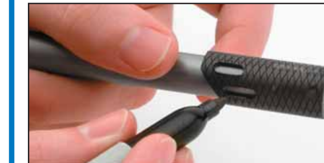
Position the Rynglok® Marking Gage (P/N: RTSG0-01-XX) on the end of the cut tube. Use a suitable marking pen to make the position and inspection marks.
