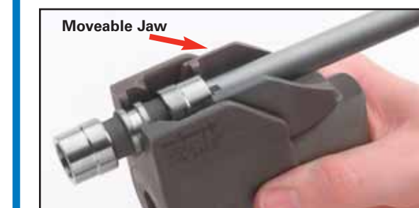
When using the tool in the forward mode as shown, position the tool onto the fitting with the tube side of the ring nested into the moveable jaw. If positioned properly, the front end of the tool will be in the fitting groove. Make sure that the fitting is bottomed into the tool.
