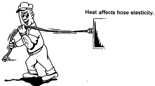
Hose failure under conditions of high temperatures plus high pressure usually take the form of early leakage at the junction of the hose and fitting. One other condition which will cause severe and rapid hardening of hose inner liner materials is the introduction of air bubbles into the fluids. This is especially true in high temperature oil systems. The entrapped hot air will oxidize and harden the inner liner tube at a rate of two to four times faster than air-free fluids.
