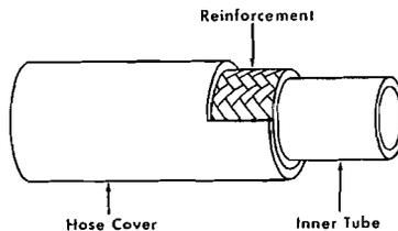
The proper selection of the hose construction to fit the application is of major importance. Generally, hose consists of three basic parts: (1) inner tube; (2) reinforcement; and (3) cover.
