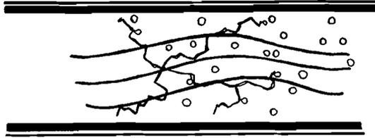
The effect of heat on Teflon hose is completely different from that of rubber hose. Unlike the more common organic rubber compounds, Teflon or "Tetrafluorethylene", as it is more properly known, does not harden when being used at elevated temperatures ( $-67^{\circ}\text{F}$  to  $+400^{\circ}\text{F}$ ), but stays uniform in texture and consistency.
