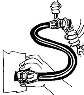
If when installing hose assemblies "common sense" precautions are observed, you will have trouble-free service. However, the human element enters when actual installations are made. Thus, the matter of individual judgment and skill on the part of technicians making the installation are very important factors.
