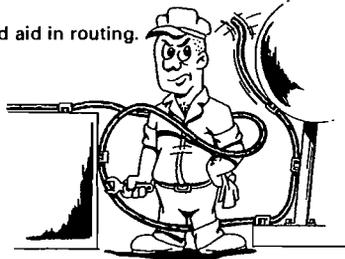
Parallel hose lines may be clamped together to improve appearance and function. Although the hose assemblies are, in a sense, operating together, each line is subject to its own impulse surges and other movements. Care must be taken so that relative movements of the assemblies will not cause the securing clamps to abrade the sleeve or hose. For example, high pressure and low pressure lines generally should not be clamped together as they tend to react differently in operation.
