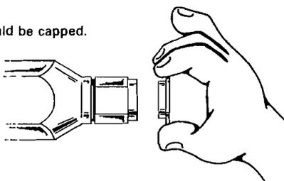
When stored, ends of hose and end fittings should be capped to prevent filtering of dirt and dust into the hose and fittings.
