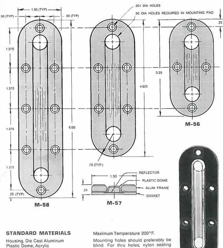
Gasket, Buna-N\* Reflector, Aluminum Alloy
