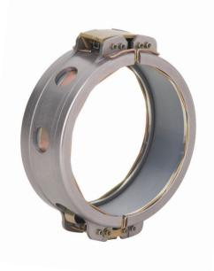
A coupling assembly general purpose is used to connect a low-pressure fluid joint by enclosing a sleeve installed over and constraining fixed cavity ferrules to create a pressure seal and electrical continuity path across the ferrules.
